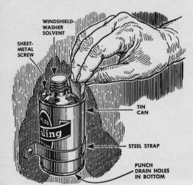
Windshield-washer solvent can be stored beside the washer reservoir by fastening a tin can inside the engine compartment with sheet-metal screws. A strip of sponge rubber slipped between the bottle and can will prevent annoying rattling.
