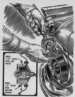
Rain water often accumulates inside the big tail-light lenses on modern cars. Locating and sealing off the spot where water enters isn't easy, but providing a drain is. Just drill two holes, as shown above, to let water out and air in.
