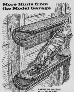
Handy storage bins for nails, screws, and small tools can be made from aluminum or galvanized steel gutters. Nail the gutters to the wall, one above the other. Use metal end caps to close the ends and to form partitions between the bins.
