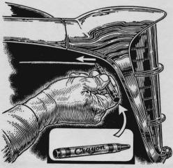
**Touch up small scratches** or paint chips with a school crayon of matching color. Rub the crayon over the scratch until it is filled. Then polish the area with a soft cloth to blend the crayon wax in with the surrounding car finish.
