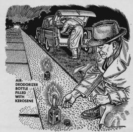
Long-burning road flares can be made by filling empty wick-type room deodorizer bottles with kerosene. When needed, unscrew the cap, pull out the wick, and light. Tightly capped bottles can be carried safely in a box in the trunk.
