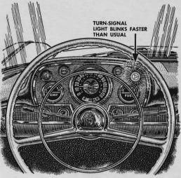
Turn indicator blinking too fast? Check your bulbs. An indicator light that blinks more rapidly than usual is the tip-off that a bulb on that side has gone out. Replacing the bad bulb will restore the indicator to its normal blinking frequency.
