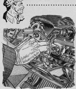
Snuff out cigarette butts safely, without taking your eyes off the road, this way: Put about <sup>3</sup>/<sub>4</sub>" of sand in the ash tray. A butt will be smothered quickly when pressed into the sand, and it can't ignite other butts in the tray.
