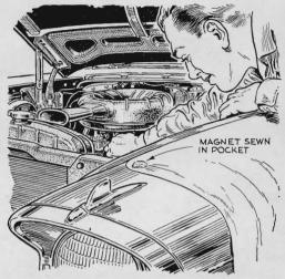
A fender cover won't slip or blow away if you sew a permanent magnet in each upper corner. Fold the corners of the cloth over the magnets, or sew a patch over them, to hold them in place and prevent them from scratching the car fininsh.
