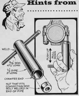
To check the big-end bearing of a connecting rod for looseness, remove one cap nut, and screw this homemade tool on the stud. The T handle affords a good grip that permits you to push the bearing up and down to detect play.
