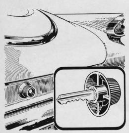
If you open the trunk frequently, you might find it more convenient to leave the key in the lock. The key can be concealed by filing its head and cementing it into a TV or stove knob. Paint the knob to match the finish of the car.
