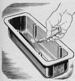
**Overhead valve noise** can be quieted by coating the inside of the rocker-arm covers with a pliable-setting gasket compound. This type of material is unaffected by the hot detergent oils that wash out other sound-deadening coatings.
