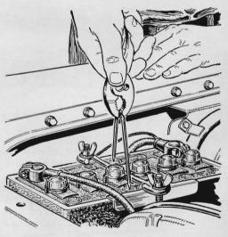
Try bridging a dead cell with the pointed ends of a heavy wire, as shown above, next time the battery won't crank the engine. Bridging the dead or open cell will often cause enough current to flow from the good cells to turn over the starter.
