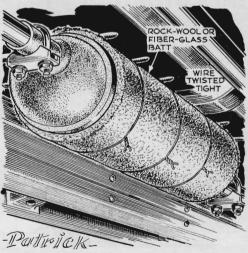
For less condensation and longer life for your muffler, wrap it with a fiber-glass or rock-wool batt to keep it from cooling too quickly. The insulation will also keep the interior of the car cooler by shielding the floor boards.
