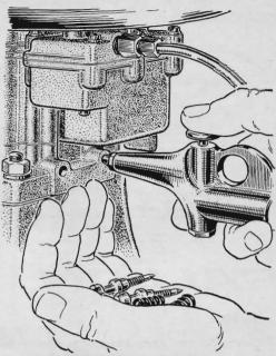
**Got a rough-idling engine?** If it can't be cured by adjusting the mixture, the trouble might be caused by dirt lodged in the idling system. Remove the adjusting screws and try blowing compressed air into the openings to clear them.
