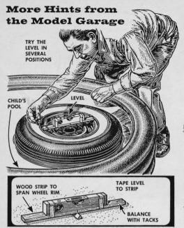
Balancing wheels precisely is easy if you float them in water. Center a level on a stick long enough to span the rim, and try the level in several positions. Add weights to the high side until the wheel floats perfectly level.
