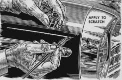
A touch-up will match perfectly if you dip a small brush in a thimbleful of lacquer thinner and rub it repeatedly over some unseen area of the finish. When the paint dissolves on the brush, apply it immediately to the scratch.
