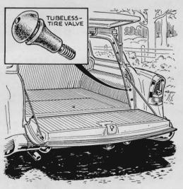
There's a use for everything—even old tubeless-tire valve stems. Drill holes in the tailgate frame of a station wagon and press the stems into them. The rounded bottom ends cushion metal-to-metal contact, effectively silencing rattles.
