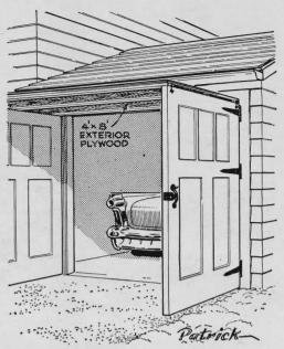
**You can gain extra room** at the rear of your garage, or shelter almost half of a second car, by extending the garage length with an overhang. Create it by fastening a panel of exterior plywood permanently across the swing-out doors.
