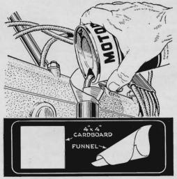
The funnel is always clean when you roll your own from a 4"-by-4" square of cardboard, manila envelope, or aluminum foil. Throw it away after using it to pour oil or fluid into the engine or transmission, and roll a fresh one next time.
