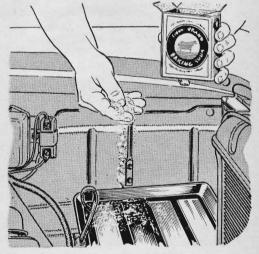
When installing a new battery, or one that's been out for a charge, brush out the metal tray of the battery holder and sprinkle some baking soda over it. The soda will neutralize any acid overflow and keep the tray from rusting.
