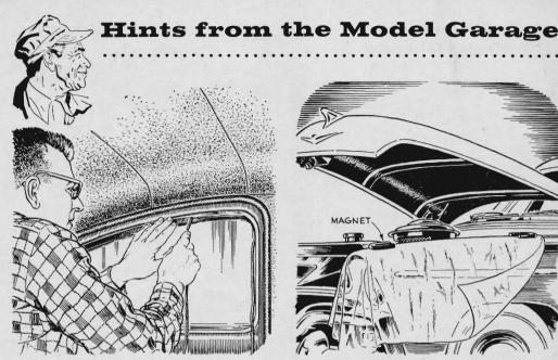
Here's a rope trick to simplify the installation of windows set in rubber molding. Place a heavy cord in the molding groove, press the window into position, and pull on the cord. The cord lifts the lip of the molding over the glass.
