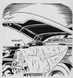
To protect your car's finish when working on the engine, drape a square of thin plastic sheet over the fender. The plastic is easy to wipe clean and folds into a tiny package for storing. Magnets make good nonslip hold-downs.
