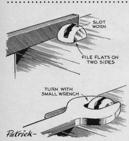
A stubborn roundhead screw that resists removal because it's frozen or its slot is chewed beyond use can be unstuck by filing flats on opposite sides of the head. Then you can use a wrench on the flats to turn the screw with ease.
