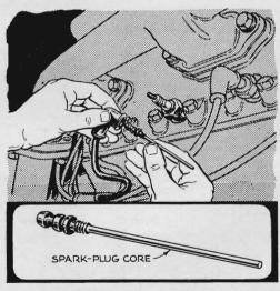
A spark tester, handy to use when spark terminals are sheathed in rubber, is easy to make this way: Break an old spark plug apart and save the core. The cap will snap easily into the wire terminal, leaving the core exposed for testing.
