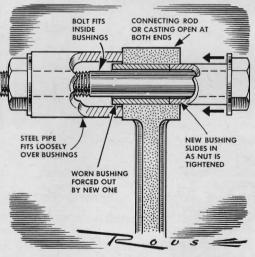
To install a new bushing quickly in any casting that's open at both ends, try the setup illustrated above. Tightening the nut causes the bolt head to pull the new bushing into the hole. At the same time it forces the old bushing out.
