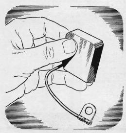
When installing new brushes in a generator, rub the corners on sandpaper to bevel them as shown. This will help the brushes to seat themselves quickly against the slightly worn surface of a commutator that has not been turned.
