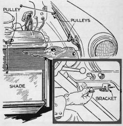
Hasten warm-up with a window shade in front of the radiator. You raise it by pulling a string run through pulleys to a bracket under the dash. Solder the pulley hanger to the front of the radiator; bolt the others in place.
