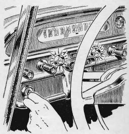
Check the lamp bulbs of your generator and oil-pressure indicator lights by noting whether they light just before the ignition key is turned to the start position. Should one fail to light, you'll know that bulb or sender is not operating.
