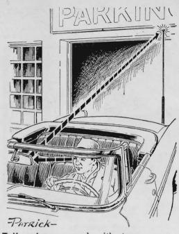
**Tall antennas** used with two-way or "ham" radios are difficult to see at night when you're passing under bridges or low-overhead openings. A bit of reflective tape wrapped around the tip will make it easier to judge clearance.
