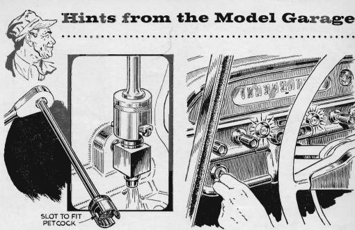
Hard-to-reach petcocks can be turned easily with an old  $\frac{9}{16}$ " or  $\frac{5}{8}$ " socket slotted and mounted on a long handle extension. Water won't run up your sleeve, either, as you open block drains. Cut the socket to fit the drain handle.
