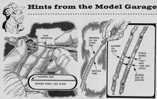
For cleaning spark plugs, a piece of spiral saw blade chucked in a drawing pencil makes a handy tool. It's especially good for scraping inside the plug. Sharpen the tip for best results. Shim the other end with tape to fit the chuck.
