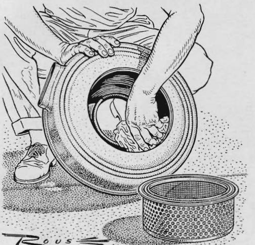
**Clean the sump, too**, when changing paper air-cleaner elements. Dirt, trapped in the sump after being stopped by the filter, may find its way into the carburetor. Best practice is to remove the whole assembly before taking out the filter.
