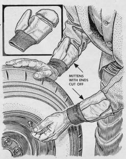
Plan ahead for roadside repairs by keeping a cut-down pair of work mittens with your tool kit. Worn upside down over your wrists as shown, the mittens will keep shirt cuffs and jacket sleeves from being soiled as you work.
