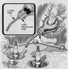
The rubber bulb from a battery or antifreeze tester can be put to other uses if the glass tube breaks. Cement a ½"diameter tube in a cork and press the cork in the bulb to make a dust blower or a syringe for adding water to the battery.
