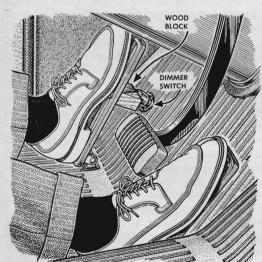
You can rest your left foot on a junked gas pedal that also actuates the headlight dimmer switch under slight additional foot pressure. Screw a wood block under the pedal to raise it to the height of the real gas pedal on the right.
