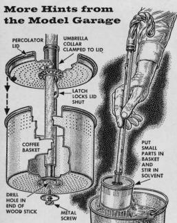
**Small-parts washer.** An old umbrella and the basket from a discarded coffee percolator are the main parts used in making this small-parts washer. Remove the stays from the umbrella collar and fit it into the percolator tube.
