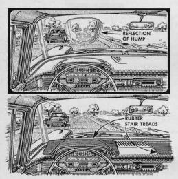
**Overcoming glare.** On some cars you get a disturbing sun reflection from the hump of the instrument panel. Draping a rubber stair tread over the hump is one way of overcoming this. A second piece can be put on the passenger side.
