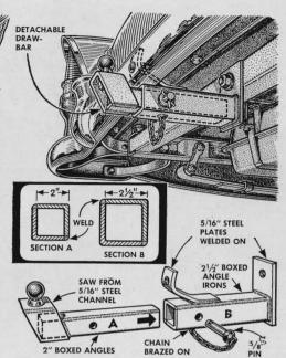
**Detachable hitch.** Here's a trailer hitch that's right there when you need it, but that's easily removed when you don't. It's best to weld up section B first, then use this as a form in making section A so that it slips nicely into B.
