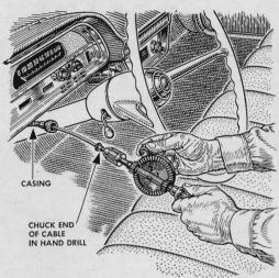
**Turn in that cable.** It's usually difficult to slide a newly greased speedometer cable back into its casing. The job is easier this way: After starting the cable, chuck the end in a hand drill. Then turn the cable as you shove on it.
