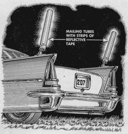
**Distress signal.** One car owner has made his own warning signals for use when he is forced to stop along the highway after dark. The picture shows how. Mailing tubes covered with reflective tape are slipped over the rear antennas.
