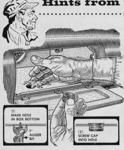
**Handy cleanout.** For easier cleaning of his glove compartment, one motorist has cut a hole in the bottom and fitted in a screw cap from a can of liquid wax. For cleaning, he removes the cap, sweeps dirt into a bag below the compartment.
