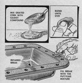
**Small breaks in cork gaskets** can be patched with a filler made by mixing grated cork with gasket compound. Grate the cork on the fine side of a vegetable grater and stir it into the compound until the mixture becomes stiff.
