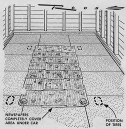
Newspapers can be placed accurately on the garage floor to catch every drop of oil dripping from the car if you mark the location of the four wheels. Since this seldom varies more than an inch or two, complete under-car coverage is easy.
