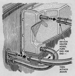
Heater hoses deteriorate twice as fast at the ends attached to the engine because of the extreme heat and oil vapor. You can double their useful life by removing them and turning them end for end when they become slightly spongy.
