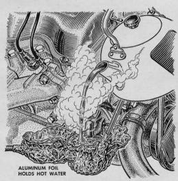
Water frozen in the fuel-pump sediment bowl is almost impossible to thaw just by pouring hot water over it. To retain the water's heat long enough to have an effect, shape aluminum foil into a container around the frozen part and fill it.
