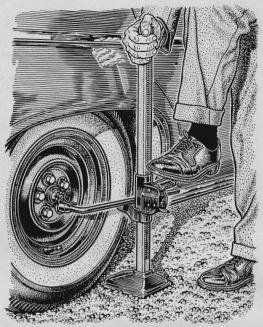
A stubborn wheel lug that resists brawn may yield to brains. Place the wrench firmly on the lug and rest the handle on the bumper jack. Operate the jack by pressing the ratchet lever with your foot until the lug loosens.
