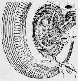
A balanced wheel should have its tire replaced in the same position—relative to the rim—as at the time of balancing. To assure this alignment, file a notch on the weighted rim and paint a corresponding spot or line on the inner sidewall.
