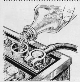
Nursing a parched battery is a cinch if you put the distilled water in an empty pint- or quart-size ink bottle. The nonspill dispensing cap (designed for filling inkwells) lets you pour without waste just the amount your battery needs.
