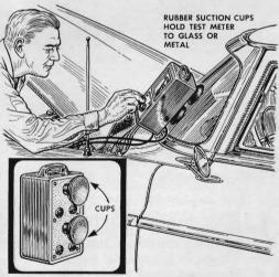
Anchor your test meter firmly in place with suction cups to prevent vibration from knocking it to the ground. You can buy rubber cups with nuts molded in them. Drill holes in the back of the meter case for bolts to hold the cups.
