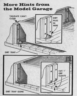
**Dirt collecting in blind corners** in the tailgate slots of a small truck or trailer often prevents the tailgate from closing fully. Eliminating these dirt traps is easy. Simply cut about 1" off the bottom of the tailgate cleats on each side.
