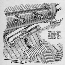
A truck fusee, besides warning oncoming motorists at night, will throw enough light to enable you to change a tire or make a minor roadside repair. Tape one or two to your car's steering post. A twist will break it loose when needed.
