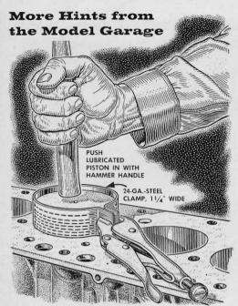
A workable ring compressor can be made from a 1½"-wide strip of steel with a tab bent at each end. Place the rings in their grooves, wrap the strip around them, and compress them by squeezing the tabs together with cam-locking pliers.
