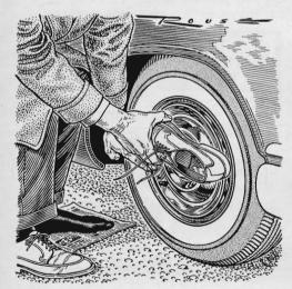
**Lacking a rubber mallet** to drive a wheel cover or hubcap into position, you can still save your hand from a bruising. Use the rubber heel of your shoe. Light blows with the shoe will seat a wheel cover in seconds without damaging it.
