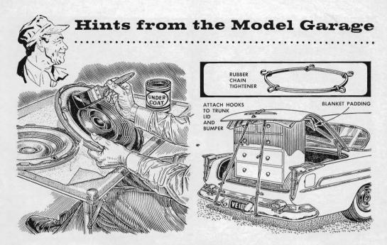
**Noisy hubcaps** can be silenced by coating the entire inner surface with body undercoating. Brush the material out to the edge of the cap and over the clips that hold it in place. This insulates the cap at all places that touch the wheel.
