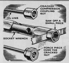
Socket Repairs Oil Line. When an oil line began to leak because of a cracked coupling nut, Norman EnHolm, of Lake Mahopac, N. Y., made an effective repair in this way. After disconnecting the union, he selected a hex socket wrench that would not quite fit on the nut. He then hacksawed a piece off the socket, squeezed the cracked nut together with a clamp, and drove on the collar. It stopped the leak.
