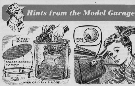
Solvent Stays Clean. Harry Morse, of Oakland, Calif., suggests putting a screen in your parts-cleaning bucket when you're taking down a unit. It lets dirt settle to the bottom and keeps it from being stirred up while you're brushing parts.
