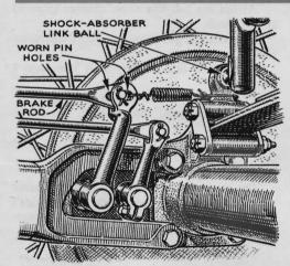
Spring Holds Brake Rod. Model A Ford owners sometimes have trouble keeping the mechanical brakes in adjustment because of worn linkages. In such cases, it's probably advisable to install new linkages if available. But you might like to try the idea illustrated above, suggested by J. O. Troemner, of Madison, Wis. The spring takes up the slack that results from the worn pin holes, preventing the brake from dragging when off.
