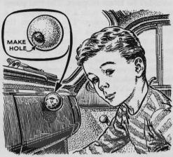
Ball Protects Children. Knobs or handles on the dash can give youngsters a bad bump on sudden stops. Sponge-rubber balls fitted over the protruding parts reduce this hazard. A dab of gasket shellac in the hole will attach the ball securely.
