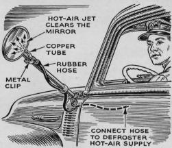
Clears Defroster Mirror. sleety weather, Ronald Weller, of Jerseyville, Ill., found that the rear-view mirror on his truck frequently became coated with ice. To keep the mirror clear, he ran a rubber hose from the defroster out to the mirror.
