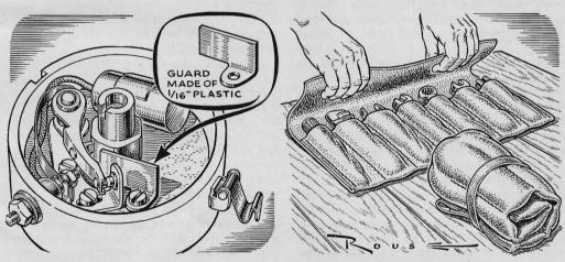
**Guard Prolongs Point Life.** Ira S. Nelson, of Chicago, reports that he has experienced considerable difficulty with burned and pitted breaker points on his '49 Ford V-8 because oil worked up the distributor shaft. As a solution, he installed a small plastic shield between the cam and breaker arm, mounting it with a 6-32 screw as seen above. The shield helps keep oil from being thrown on the points.
