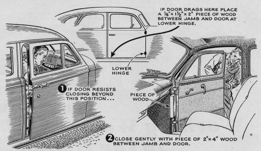
Repairing Sprung Doors. Unless they are too badly damaged, doors with sprung hinges can sometimes be put back into working condition by deliberately jamming them against a piece of wood. Burk Jaggers, Rushville, Ind., writes that he has used the method above. In closing the door, always proceed gently and keep testing—or you may have the problem of correcting an overcorrection. Should the door rub at the upper rear corner, place your block of wood between jamb and door at the top hinge.
