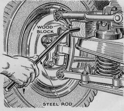
Block Stops Wheel Sag. If you've ever used a bumper jack, you've probably noticed that the front of a car must be raised quite high before the tire is free. This is because the suspension arms allow the wheel to sag. You can overcome this by thrusting a block of wood between the frame and upper wishbone. A block cut from 3" by 3" stock will do the job. To position the block, fit a steel-rod handle into it.
