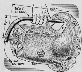
**Transmission Lifter.** Back in the days when Fords had the shift lever on the floor, the lever could be used to lift the transmission out of the car. But on later models there's practically nothing to which you can hold. To ease the job, mechanic William E. Ware, of Shirley, Ind., made the lifter shown here.
