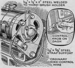
Varies Generator Output. This control enables Rowlins Howard, Rushville, Ind., to vary the generator output on his 1934 Chevrolet to suit conditions. On short hops and at night, he pulls the knob and gets readings of 15 or 20 amp. On a long trip he cuts output back to 4 or 5. This helps prevent battery overcharging.
