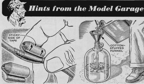
Look, One Hand! In a spot where there's barely space for one hand, how can you tape a wire? Simple enough, says Harry Morse, Oakland, Calif. Tear off a piece, re-roll with the sticky side out, and wind on with the fingers of one hand.
