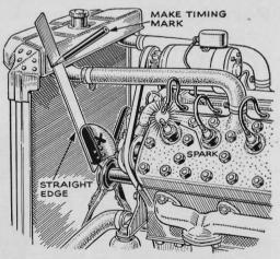
**Ignition Timing Kink.** Here's an easy method, writes H. W. Mills, of Albion, Ill., for checking the timing of a car with a direct-drive fan. Slowly crank the engine with the ignition on after disconnecting No. 1 spark plug. When you get a spark, use a straightedge on a fan blade to mark a spot on the radiator. Also identify the fan blade as well. This is mainly useful if one mark is made when the timing is just right.
