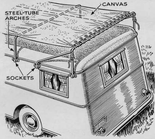
**Awning Shades Trailer Roof.** The interior of a parked trailer often becomes unbearably hot when the summer sun beats directly on it. To remedy this condition, A. V. Malone, of Los Angeles, built the shade shown above. It's canvas stretched over steel tubes that fit into sockets on the trailer. Mounted about 12" above the roof, it has open sides for air circulation, lowering the inside temperature 10 to 20 deg.
