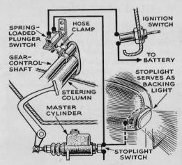
**Light for Backing Car.** F. W. Atwood, of Danvers, Mass., wired his stoplight so it serves also as a backing light. He mounted a spring-loaded switch on the firewall and a hose clamp on the shifter rod. Shifting into reverse turns on the stoplight. It's wired through the ignition so the car can be left parked in reverse. The motor can be started without the key (with shift in reverse and brake on), but this does no harm.
