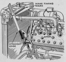
**Ignition Timing Kink.** Here's an easy method, writes H. W. Mills, of Albion, Ill., for checking the timing of a car with a direct-drive fan. Slowly crank the engine with the ignition on after disconnecting No. 1 spark plug. When you get a spark, use a straightedge on a fan blade to mark a spot on the radiator. Also identify the fan blade as well. This is mainly useful if one mark is made when the timing is just right.
