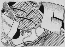
Floor Pads Stop Drafts. that blows in around the shafts of the clutch and brake pedals can be stopped by pieces cut from an old inner tube or step pad. F. W. Marasco, of McKeesport, Pa., writes that it isn't necessary to secure the slit pieces if you cut them large enough,
