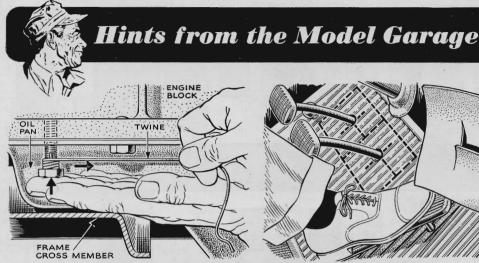
Twine Starts Bolts. Ben H. Clare. of Wellsville, Mo., suggests you use twine the next time you have to start a bolt in a hard-to-get-at spot. Wrap the bolt with twine, hold it in place with a finger or screwdriver and pull the twine. Sometimes it may be necessary to taper the end of the bolt.
