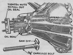
Bolts Pull Oil Retainer. The oil seal on the differential housing of one Plymouth seemed to be in for good, but Stanley T. Lusas, Woodbury, Conn., found a way out. Sawing a flat on two 3/8" carriage bolts, he was able to slip the altered boltheads into the groove from which the felt ring was removed. By alternately tightening nuts against a simple bar voke, he drew out the seal. Different bolts may be needed on other cars.
