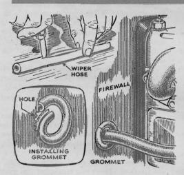
Grommet Guards Heater Hose. In making a hole in the firewall for heater hose you may have to drill a circle of holes and chisel out between them. Protect the heater hose from the jagged edges by slitting a piece of windshield-wiper hose and cementing it around the rough inside edge.
