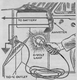
Trouble Light Doubles in Car. One extension cord kept in the car is always available for use as a trouble light with the accessories added by W. M. Dierks, of Chicago. He installed a standard 110-volt outlet in the car, wiring it from the ammeter to ground. At the other end is a 6-volt bulb with a standard screw base. For use on house current it is only necessary to replace the bulb with a 110-volt one.
