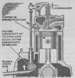
Wear Alters Clearance. Worn camshaft bushings may cause burned valves by reducing the apparent tappet clearance. Caral Lee, of Weld, Me., suggests this test for Chevrolets: Set the No. 1 tappet, remove the fuel pump, pry up the camshaft, and recheck the clearance. Since the camshaft tends to ride at the top of its bushings during rotation, the measured difference should be added to the normal clearance.
