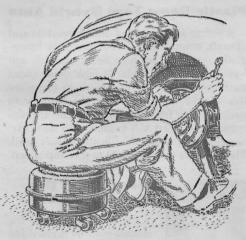
stool Built of Brake Drums. One mechanic made his job easier by welding two discarded brake drums together. Four casters on the bottom and a sheepskin buffing pad on top make it a serviceable rolling stool. It's particularly good for jobs for which you'd ordinarily have to kneel.
