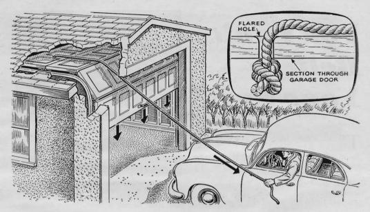
**Rope Closes Overhead Door.**With this arrangement, you don't have to get out of the car to close the door after leaving the garage. Just grab the rope dangling near the jamb, and give it a pull after you have backed out. Attach the rope (a
