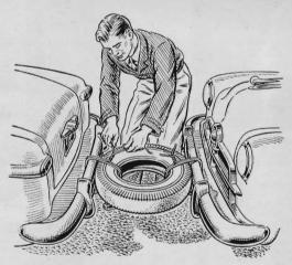
Tire Cushions Towing Bumps. An old tire makes an excellent coupling to a car that you want to tow. Pass a few turns of heavy wire or rope around the tire and the respective bumpers of the two cars and you are ready to go. The tire effectively smooths out the jerks and nicely cushions the bumps in stopping, writes Leslie H. Housel, of Grass Lake, Mich.
