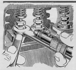
Light on the Spot. Adjusting valve tappets on a car is a fussy job to do just right. What makes it troublesome is the necessity of manipulating wrenches and a thickness gauge in cramped quarters with inadequate light. Albert S. Eaton, of Belmont, Mass., reports that the work goes a little easier if you tape a pocket flashlight to the upper tappet wrench.
