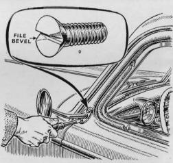
Filed Screws Prevent Theft. If you attach a mirror, road light, or other accessory with external screws, safeguard it against theft by filing off those corners of the slots that the screwdriver bears against during removal. Once tightened, the screw is next to impossible to remove, so use it only on permanent installations. You can retighten it, however, if vibration loosens it,
