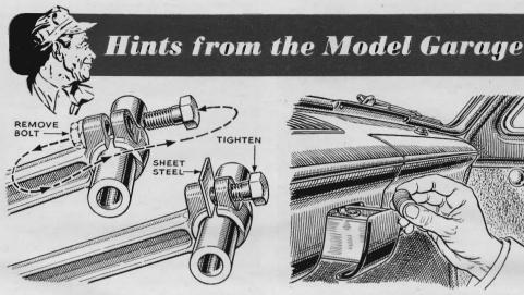
Con Rod Pressed Open. Wrist pins to be clamped in connecting rods of the kind shown will not always go in easily, even with the bolt loosened. If assembly proves difficult, reverse the bolt as shown and use it and a piece of thin steel to spring open the con rod very slightly. Replace the bolt in its proper position after doing this.
