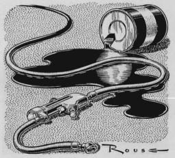
**Oil Rots Rubber.** If you run a shop, you know the cost of air hoses, battery-charger cables, and other rubber equipment. One sure way of increasing this cost is illustrated here. Grease and oil cause rubber to disintegrate rapidly. So keep such equipment off the floor. It's also a good idea to wipe off the lines occasionally.
