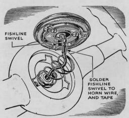
Swivel Safeguards Horn Wire. In some cars the horn wire inside the steering column is subjected to considerable twisting. C. B. Hopkins, of Tacoma, Wash., found that this caused the wire on his 1941 Ford to break several times. A brass fishline swivel, taped as shown above, took care of the problem nicely.
