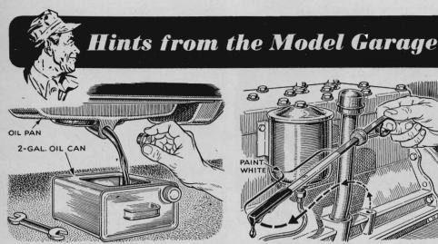
Oil Drained into Flat Can. Some new cars are so low that it's awkward to drain the crankcase without a lift. The job calls for a shallow but capacious pan. Victor H. Lamoy, of Upper Jay, N. Y., reports that an empty 2-gal, oil can with a large opening cut in one side gets under easily. Leave a lip around the hole to keep the oil from slopping when you drag out the filled can,
