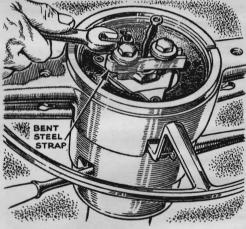
**Steering Wheel Puller.** Removing the steering wheel of a Frazer without damaging the wire to the horn button was a problem until I hit on the simple puller illustrated here. It is a piece of %" by %" steel strap bent to a U-shape. Two bolts, supported by washers, were used to pull the wheel. Of course, the nut on the steering post was loosened, but not removed, to provide a bearing surface for the U-bracket.
