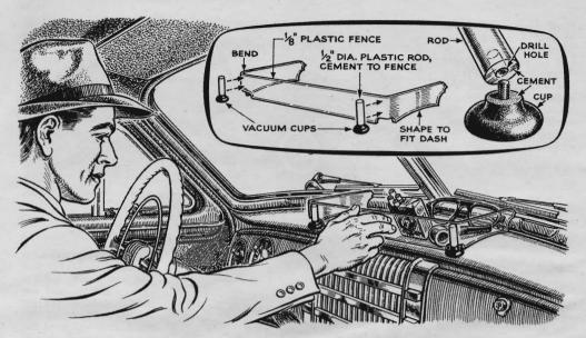
**Dashboard Fence of Plastic.** A strip of %" plastic, bent and cemented to two posts, forms a dashboard fence that will hold a lot of those miscellaneous items you frequently need while driving. Small vacuum cups cemented and threaded to the rods will
