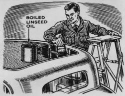
Linseed Oil Dresses Fabric Top. I have found that a good dressing for fabric tops is boiled (not raw) linseed oil. It even seals small leaks in the top, and does not crack because it is flexible. However, it requires considerable time to dry. Any paint store has it, but be sure it is boiled linseed oil.-G. E. Boud, Youngstown, Ohio.
