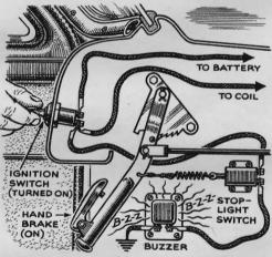
**Buzzer Warns Hand Brake Is** On. After catching my wife driving with the hand brake on for the third time, I devised this simple warning gadget that is similar to those found on newer cars. I connected a doorbell buzzer through a stoplight switch to the ignition switch, as shown in the drawing. Turning the key sounds the buzzer until the brake lever is released. The buzzer is under the dash.-W. M. Dierks, Chicago.
