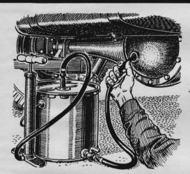
Can Makes Pressure Filler. A 2or 5-gal. can, with a tire valve soldered in the top and a petcock soldered in the side near the bottom, makes a pressure filler for auto differentials and transmissions. Attach a flexible hose to the petcock and put a few pounds of air through the valve with a hand pump or air line and the filler is ready for use. The same idea works on a 55-gal, drum for dispensing bulk liquids.
