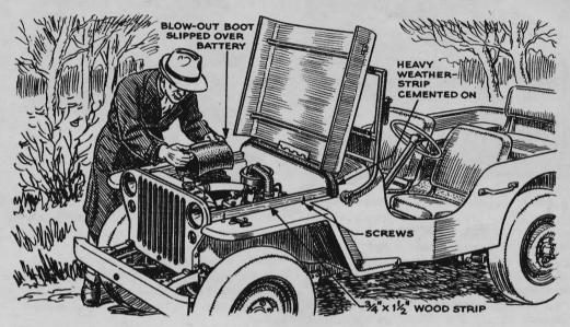
**Jeep Engine Kept Dry.** David Horvath, of Yonkers, N. Y., writes that he frequently had trouble starting his Jeep because water and snow collected around the spark plugs and on the battery and wiring. This sketch shows how he waterproofed the en-
