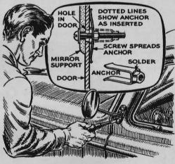
**Toggle Nut Holds Mirror.** When the original self-threading metal screw tore loose, B. Leo DeMare, of Aberdeen, Md., devised the nut shown above to fasten a rear-view mirror to his car. A nut first was filed down slightly to clear a hole in the door frame. A strip of sheet brass was drilled, soldered to the nut and bent into a U. The nut and anchor were threaded on the bolt, inserted in the hole, and drawn up tight.
