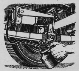
Shocks Filled with Oil Can. Here's a rig that will enable you to refill shock absorbers without difficulty when the filler plug is located in a hard-to-reach spot. Suggested by Marion L. Rhodes, of Knightstown, Ind., it consists of a pump-type oil can, a length of rubber tubing, and a small nozzle bent from copper tubing. With the nozzle inserted, a few strokes on the pump handle will quickly refill the shock.
