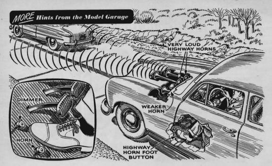
Horn Button on Floor. As a safety measure—so I can keep both hands on the wheel when I'm driving fast—I mounted an auxiliary horn button on the floor of my car. For this button, I used a floor-type starter switch. I located the switch near the dimmer
