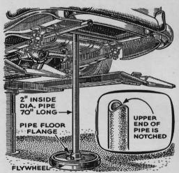
Stanchion Opens Springs. I really get oil between spring leaves with this stanchion. After the notched upper end is placed under a frame cross member, I lower the lift a couple of inches. This takes some of the load off the springs and the leaves open. You can almost pour oil between the leaves .-Marion Rhodes, Knightstown, Ind.
