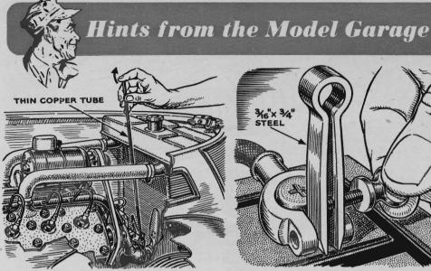
Copper Tube Makes Oiler. To get at those hard-to-reach oil fittings, try this: dip some copper tubing about an inch into oil. Trap the oil in the tube by pressing your finger over the upper end. Removing your finger releases the oil in the fitting.
