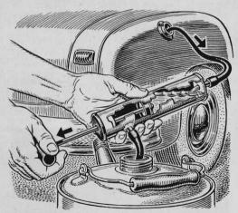
**Spray Gun Siphons Gas.** A siphon for drawing gas from a tank can be made out of an insect spray gun. Take out the plunger and reverse the cup leather. Cut off the spray container, enlarge the hole in the end of the cylinder, and solder in a piece of 4" copper tubing. Solder a delivery tube near the other end.
