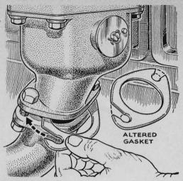
Gasket Slots Ease the Job. Narrow slots cut from the edge of a gasket to the bolt holes allow you to install a new one without taking out the bolts. This may be specially helpful on exhaust manifolds or other parts where bolthead clearance is scant, or where threads are so rusty that complete removal would be a time-consuming job. Just loosen the bolts enough to separate the flanges. The slots do not impair the efficiency of the gasket.
