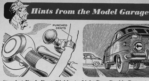
Steering Knob Kept Rigid. spinner knob that twists in or out on the steering wheel can be cured by putting a few punch dots in the clamp. To avoid the possibility of cracking a plastic wheel, it's best to remove the spinner and clamp it on a broom handle or similar object. With a prick punch, make four or five dimples on opposite sides of the strap. When clamped, the spinner will remain in position permanently.-Jim Sisley, Seattle, Wash.
