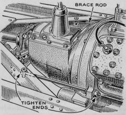
Keep Support Rods Tight. On prewar Ford V-8s, the two support rods that help anchor the engine at the rear have sometimes led to a false diagnosis of clutch trouble. If the rods loosen up, the result is similar to clutch chatter. The remedy is simple: either tighten the rods or replace them.-A. Zanelli, Clifton, N. J.
