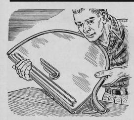
Replacing a Skirt Gasket. You can use a wide washing-machine cover gasket to replace a worn one on the fender skirts of some cars. Cut the rubber to length and stretch it around. Run a small wire hook through the inner side of each end. Fasten the hooks to the projections on the back of the skirt to hold the gasket.
