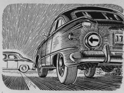
Light Does Double Duty. An accessory back-up light-the kind controlled by a separate switch—can be put to extra use as a direction indicator. Using red paint, I painted on the lens a big arrow pointing to the left. Now, when I'm making a left turn or pulling away from the curb, I flick the light on and off a few times. I've used the light for some time now and find it does its new job very nicely. It still gives ample light for backing.-Ray Smiley, Detroit, Mich.
