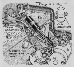
Short Lead Improves Starting. On an older-model Plymouth, I have found that moving the coil from the firewall to the spark-plug cable support makes the engine easier to start. In the new position, the high-voltage wire from the coil to the distributor cap is shortened considerably.—Ralph Wyant, Indianapolis, Ind.
