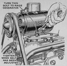
Tool Supports Generator. On some cars it's very tough to hold the loosened generator up in position while adjusting belt tension. The tool illustrated takes care of this. It consists of a piece of ½" steel plate tapped for four ½" bolts. Turning the one at the center with a wrench gives a powerful upward thrust, holding the generator at the desired level until the belt-adjustment nut can be tightened. Adjust the length of the leg bolts as required.
