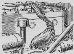
Sleeve Protects Ignition. If you have had trouble with the ignition shorting out during heavy rain, here's an idea that may help you. Cut an 8" section from an old inner tube, snap loose the distributor cap, slip the rubber sleeve over the high-tension wires, and replace the cap. Draw together and tie the sleeve at the topmost edge.
