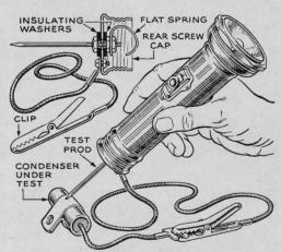
Flashlight Tests Circuits. A flashlight with a metal case makes a good continuity tester. Rufus P. Turner, of New Bedford, Mass., rigged this one. The test prod is a 3" brass rod threaded for 6-32 nuts and insulated from the cap by fiber washers. The other lead runs directly to the cap. In use, the bulb lights to indicate grounds and shorts. No light shows on an open circuit or an unshorted condenser.
