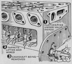
Clothespins Wedge Valves. Here's a time-saver in removing the camshaft of an L-head engine: Instead of removing the valves, springs, and tappets, just raise each valve spring with a valve-spring lifter and wedge a clothespin or piece of wood under the valve head. Then lift and wire each tappet up out of the way. The thrustplate then can be removed and the shaft pulled out. Kaiser-Frazer Corp. suggests this.
