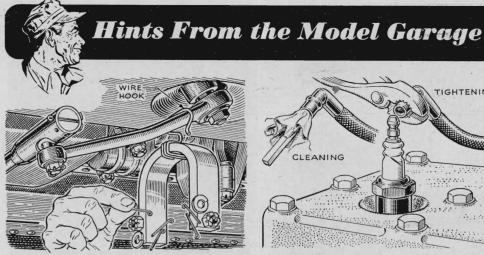
Magnet Holds Small Parts. When you're working under a car, hook a permanent magnet nearby. As you remove nuts, cotter keys, pins, or small parts, just stick them to the magnet. P. R. Wilson, of Brooklin, Ont., says this is a help when you replace the parts. They're right there when you want them, and they don't pick up grit.
