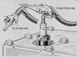
Dirty Cap Causes Miss. On highcompression engines, mysterious low-speed missing or bucking may sometimes be traced to poor electrical contacts in the high-tension leads. According to Frank Tobin, of Manhattan, N. Y., cleaning out and tightening the plug caps will often cure skips seemingly caused by defective plugs,
