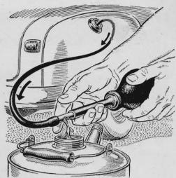
**Syringe Used as Siphon.** Neoprene tubing, a short piece of copper tubing, and a syringe may be quickly assembled to siphon gas from a car. File a half-round hole in the copper. To use, compress the syringe bulb, place your thanb on the hole, allow the bulb to expand, and uncover the hole. Remove the syringe when gas starts.
