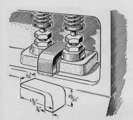
Tool Simplifies Valve Work. Here's just what the doctor ordered for admasting Kaiser valves. Machined to an exact width of ¾", the tool slips between the flats of adjoining cam followers. This jams them, leaving your hands free to make the adjustment. The longer arm is filed to ¾" thickness. A. G. Patrick, of Hot Springs, Ark., made the tool when he found there wasn't space for a conventional wrench.
