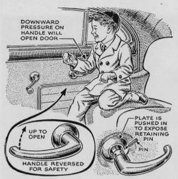
Children Can't Fall Out. In some cars, the handles are pressed down to open the doors. This is a hazard, since any rider, especially a child in the back seat, may lean on the handle and open the door by accident. S. W. Trosell, of Manhattan, N. Y., found a simple solution for this. He reversed the handles.
