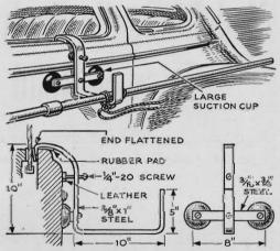
Brackets Carry Pipe. If you sometimes must carry long lengths of pipe, lumber, or other materials on a car, a pair of removable brackets like this will make the job easier and prevent the finish from being scretched. A ½"-20 screw clamps the flattened top end of the bracket to the car. Use at least ½" steel, or heavier if possible. When the brackets are complete, give them a coat or two of paint.
