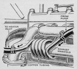
Heater Output Boosted. John P. Berkyta, of Lyndhurst, N. J., writes that the hot-water heater in his car failed to provide the warmth he likes. He solved the problem by making use of some of the heat that's wasted out of the exhaust pipe. Taking a length of copper tubing, he wrapped it several times around the exhaust manifold, connecting one end to the heater and the other to the pump.
