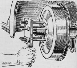
Stubborn Wheels Come Here's a wheel puller devised by Raymond Holtz, of San Francisco. It consists of a square of ½" steel plate and five studs. Five holes in the plate match those in the brake drum. One end of each stud is threaded to go into the brake-drum holes, the other to take a standard nut. In use, the nuts are tightened alternately. Pressure against the axle pulls the wheel.
