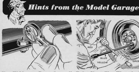
Key Hidden on Dress Snap. If you'd like to keep an extra gas-cap key hidden in your car, here's one way of doing it. Solder half of a dress snap to the key, the other part to the head of a small bolt. Then insert the bolt in any convenient hole-in the dash flange, glove compartment, or other place where the key will be out of sight.
