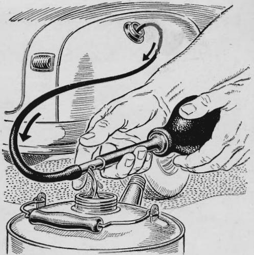
**Syringe Used as Siphon.** Neoprene tubing, a short piece of copper tubing, and a syringe may be quickly assembled to siphon gas from a car. File a half-round hole in the copper. To use, compress the syringe bulb, place your thumb on the hole, allow the bulb to expand, and uncover the hole. Remove the syringe when gas starts.
